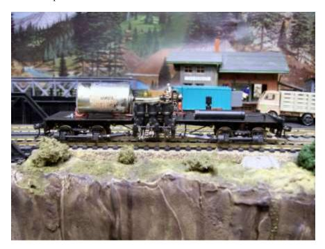
The superstructure was missing the front bolster and steps. I found a plastic one in the junk box and glued it on. Kadee couplers were added. A rear headlight was purchased from Custom Railway Supply. I still haven't done anything with the headlight or stack screen. Careful application of flat black from a 'rattle can' produced good results. I also painted the interior to eliminate brass shine. The locomotive was reassembled, and runs well. Shays are NOISY! Don't think I'll try to install DCC.
