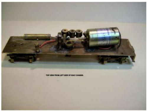
After extensive working, the chassis moved on DC. Application of "Darken-it" didn't darken the chassis parts, so I resorted to brush painting. I applied paint to the top of the chassis, the cylinders, truck frames, and any other parts that wouldn't interfere with operation. The result is shown here.
