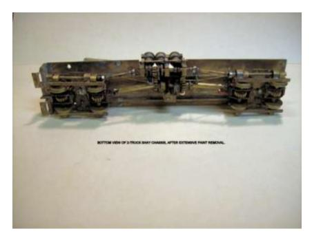
With the motor re-installed (It was a replacement can motor from Wayne Lemle's store sometime in the past, for \$17.95) I placed the chassis on the track and tried it out. Motor ran, mechanism tried to move, but jammed. Then the tubing started slipping on the drive gear. A shot of "super glue" stopped the slipping, but the mechanism still didn't want to turn. I banged on it some more.
